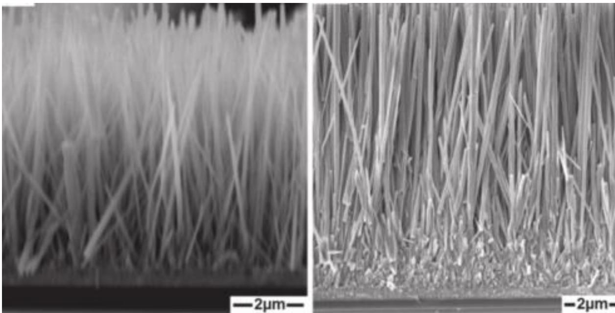
Cao, G., Hong, K., Wang, W., Liu, L., & Xu, M. (2016). Fast growth of well-aligned ZnO nanowire arrays by a microwave heating method and their photocatalytic properties. *Nanotechnology*, 27, 435402–7
